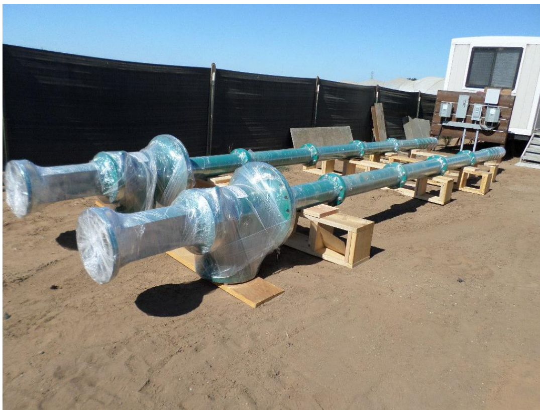
Vertical turbine pumps delivered to site.
