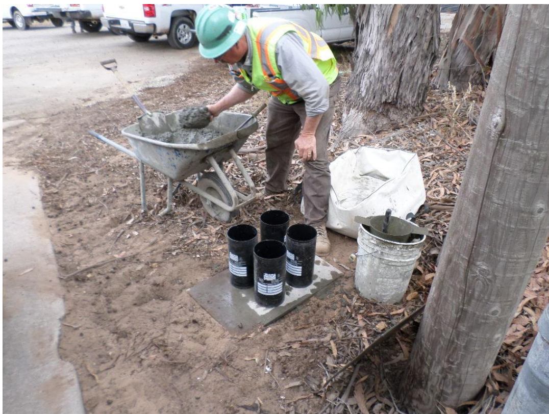
Fugro taking concrete test cylinders.
