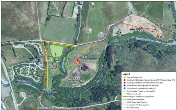
Figure D-4. Cambria CSD Desalination Schematic
