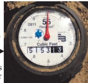
Subtract Read #1 from Read #2 (515313-514828); this equals the cubic feet used (485). Multiply this number by 7.48 to get gallons used (3,627).
