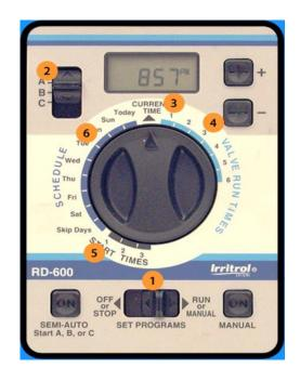
The **Run Time or Station Duration** is the time (in minutes) a specific valve will stay open and provide water to a zone.
