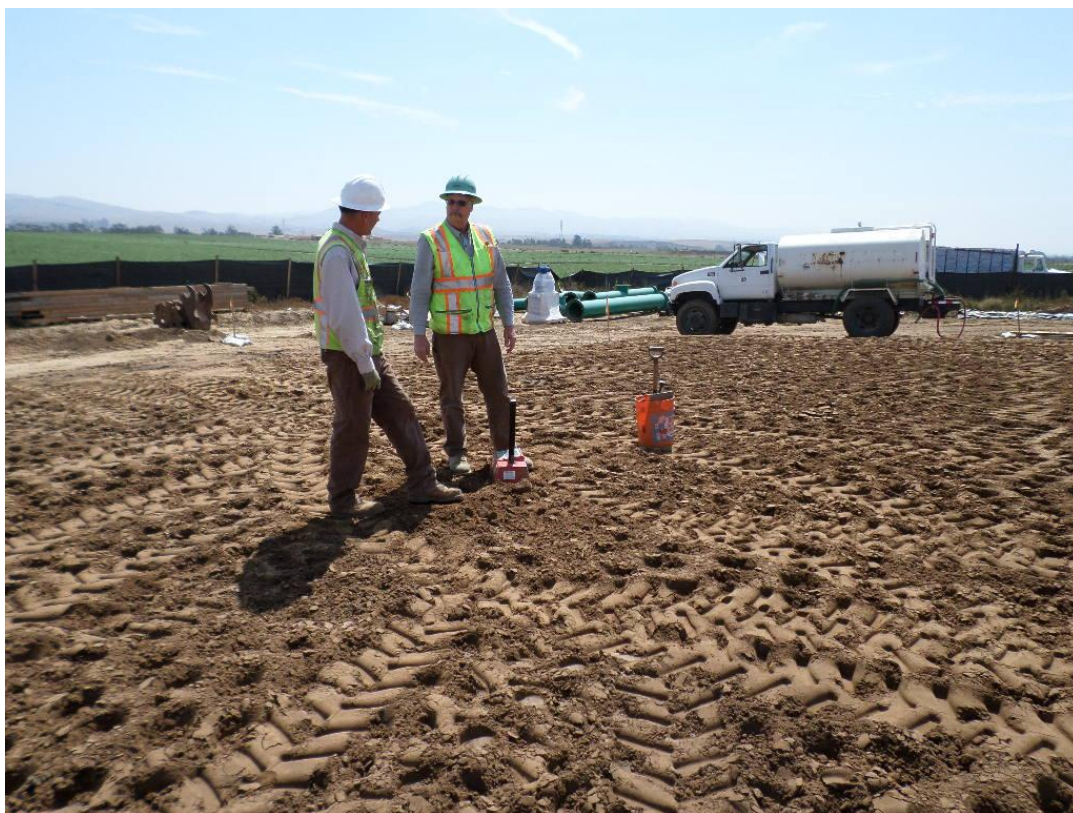
Fugro on site to test compaction of backfill at future pump station.
