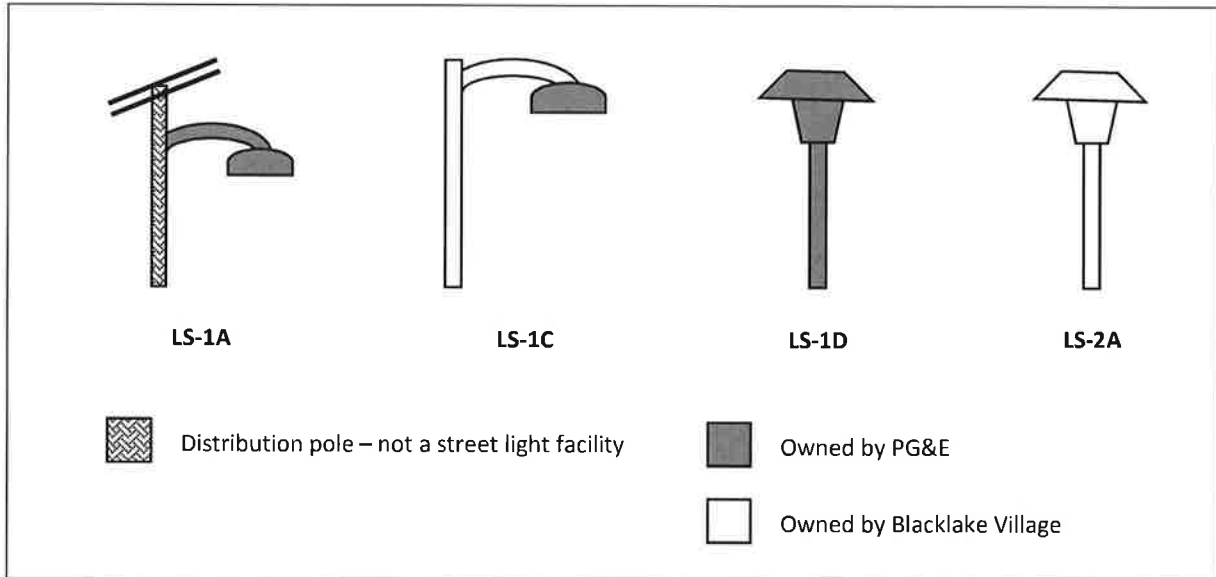
Figure 1: Ownership of Blacklake Village Street Light Facilities by Tariff
