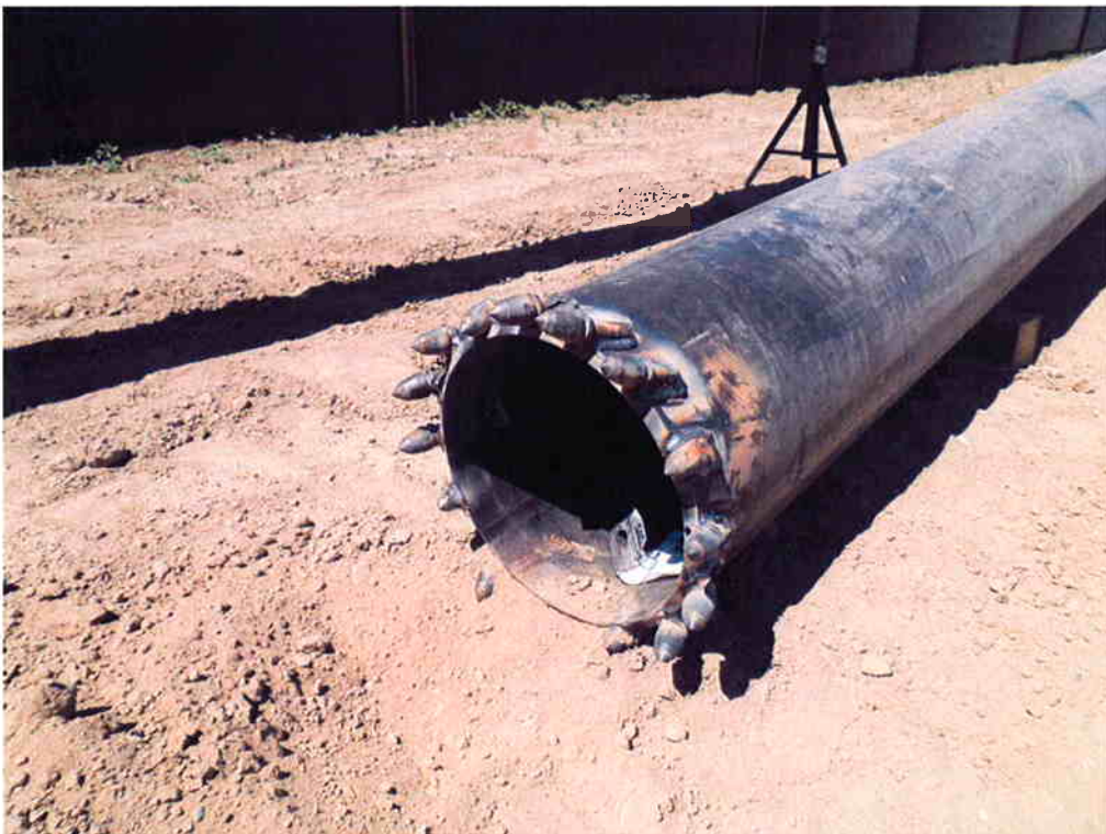
Steel "teeth" welded onto the end of the 12-inch casing to assist with installing it.
