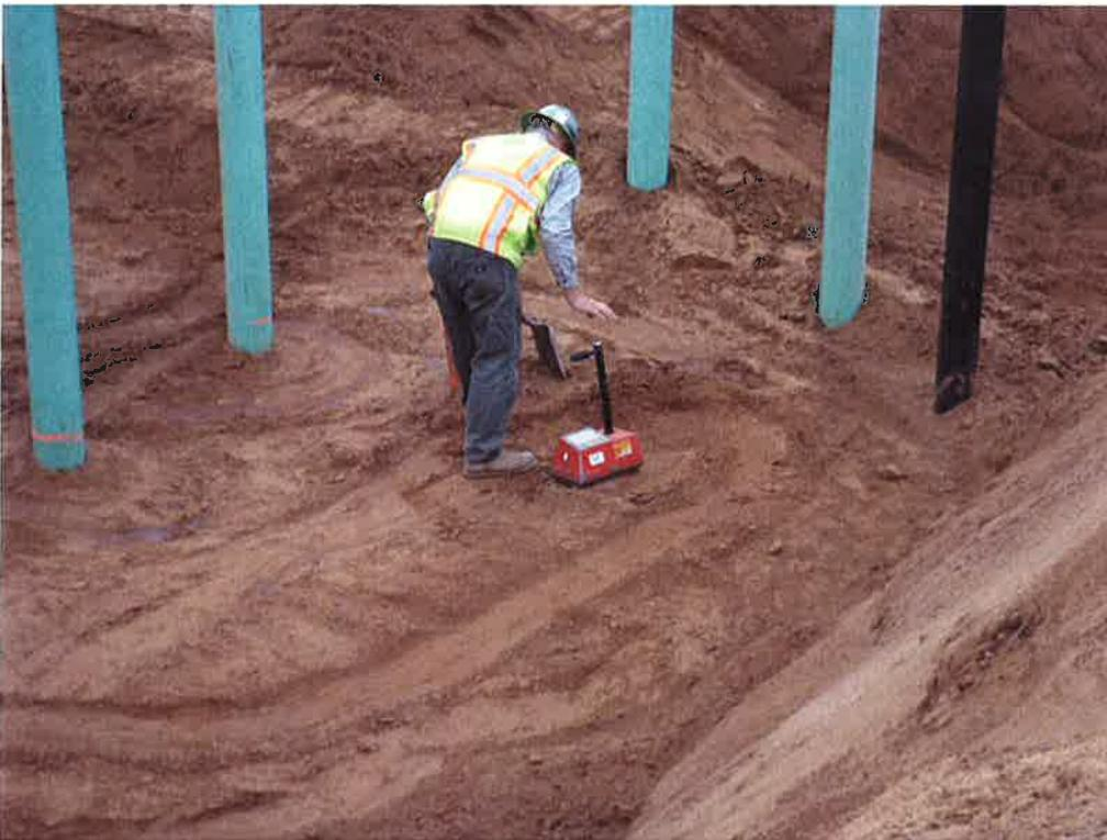
Fugro testing compaction.
