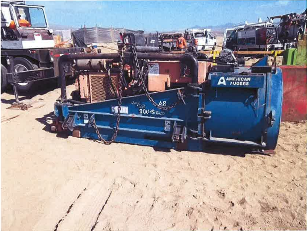
Bore and jack machine mobilized to the site by Pacific Boring.
