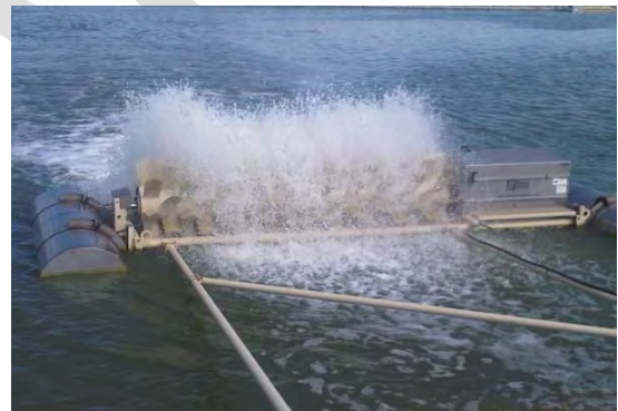
House Brush Aerator with Levee-stake Anchoring
