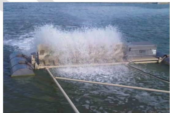
House Brush Aerator with Levee-stake Anchoring
