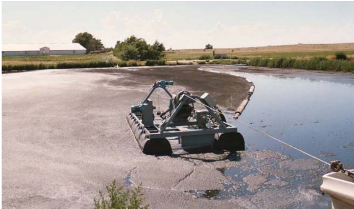
Figure 7-5 Severe duty Flump® operating on traverse system to dredge a pig lagoon
