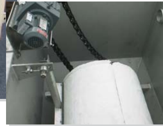
Internal view of AquaDrum™ filter.
