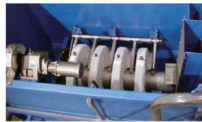
Internal view of 4-disk Aqua MiniDisk™
