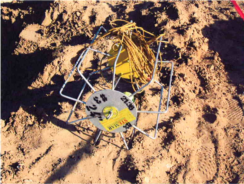
Mandrel used for testing the 24" SE2 pipe.
